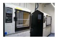
Alternating condensation climate test containing sulphur dioxide (Kesternich) according to DIN EN ISO 22479 / DIN EN ISO 6988 / DIN 50018
